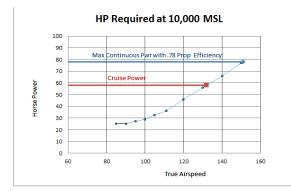
Note the chart above the engine HP available and required actually are very precise. This allows you to optimize your cruise. A line from Zero airspeed to the tangent of the line yields the exact max cruise speed for maximum range.
