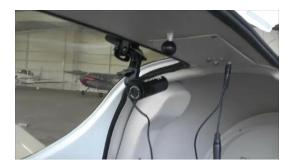
Post flight review of the video will reveal instrument readings, but also the running video time will verify climb rate and the test point accuracies.
