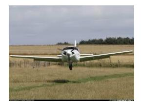
The normal or short field landing pattern should be planned to enter at the speed identified in the POH. In absence of manufacturers guidance, use the flap limiting airspeed.
